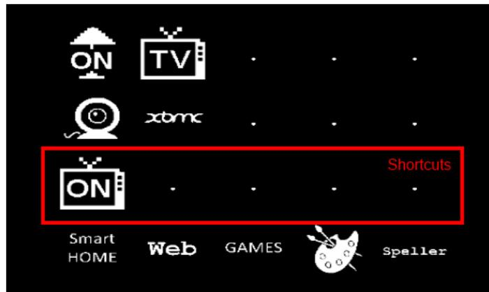
**Fig. 5** Interface interaction to turn the TV on when the corresponding shortcut is suggested by the system.
