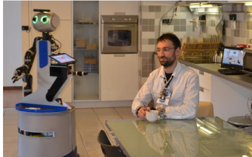
Fig. 5. Domocasa Lab – IT, the robot reach the user in the kitchen and acted as a physical reminder
